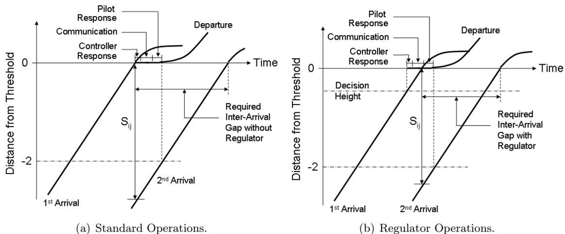
Figure 1: Diagram of Closely Spaced Parallel Runway Operations under IMC
